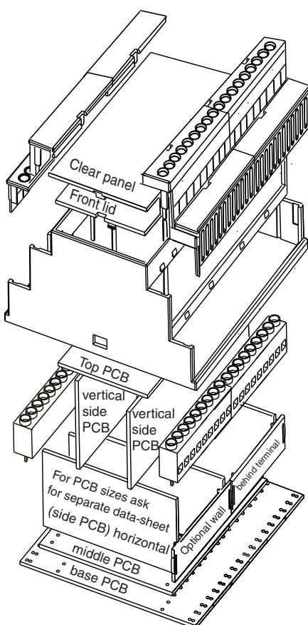
With the advantage of the building block method you can flexibly build your own DIN-rail enclosures with the option of printed circuit boards with terminals on two board levels.
